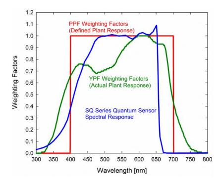
Radiation weighting factors for PPFD (defined plant response to radiation), YPFD (measured plant response to radiation), and Apogee SQ Series quantum sensors (sensor sensitivity to different wavelengths of radiation).
